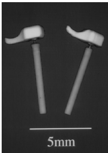
Fig. 39. Ossicular replacement prostheses. Head of the prosthesis is synthetic HA, and the stem is a bioactive composite of HA particles in a polyethylene matrix. (Photo courtesy of Professor Bill Bonfield and Dr. Elizabeth Tanner.)
