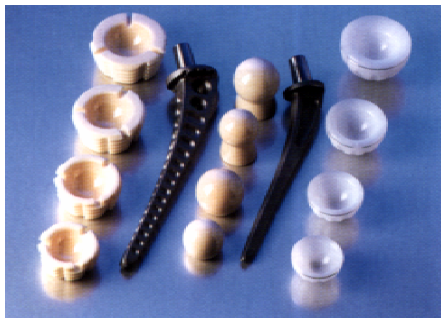
Fig. 7. Medical-grade \text{Al}_2\text{O}_3 used in total hip replacement: (left) \text{Al}_2\text{O}_3 acetabular cups mated with \text{Al}_2\text{O}_3 femoral balls; (center) \text{Al}_2\text{O}_3 balls also can be used with ultra-high-molecular-weight polyethylene cups; and (right) alternative metallic stem designs for morphological or cement fixation. (Photo courtesy of Dr. Gerd Willmann, CeramTec AG.)
