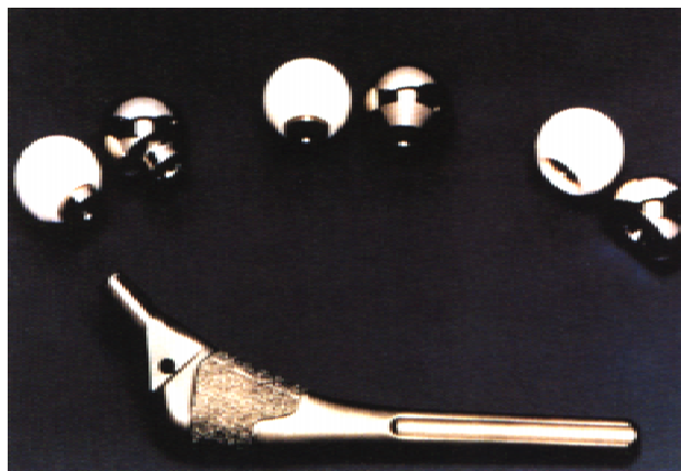
Fig. 8. Medical-grade \text{Al}_2\text{O}_3 used as femoral balls in total hip replacement. Note the porous coating on the metallic stem used for biological fixation. (Photo courtesy of Dr. Jack Parr.)
